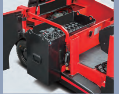
The Tow Tractor features the battery side roll out feature standard in order to replace the battery fast and easy.
