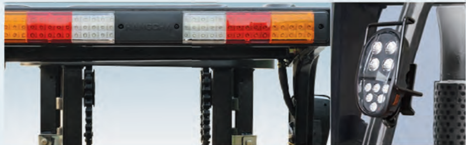
The new efficient lighting system uses LED's and a new type of reflector to reduce energy consumption. This significantly improves illumination performance while also prolonging operation time.
