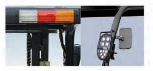
The new efficienct lighting system uses LED's and a new type of reflector to reduce energy consumption. This significantly improves illumination performance while also prolonging operation time.
