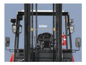
The mast was redesigned to provide broad forward visibility. This was done by increasing the distance between inside mast by 2.34"
