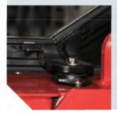
Dampening pads are placed where the chassis meets the steering axle, engine, torque converter, and the overhead guard. The suspension seat also comes standard. This is all included in the design to reduce the amount of vibration to the operator and increase operator comfort.
