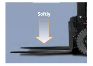
In addition to the soft landing system, the soft lifting system is adopted (front lifting cylinders of the full free lift 2 & 3 stage masts). As a result, the noise and shock of the mast significantly decrease when lowering materials.
