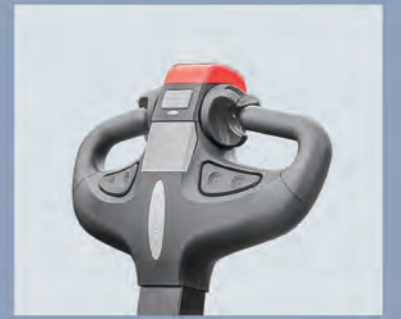
The ergonomic tiller head allows for easy operation with one hand.
