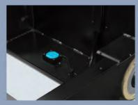
The tilt sensor prevents the vehicle from tipping over due to excessive slope and ensures operator safety.
