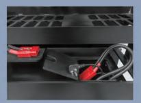
Battery side roll out and built-in charger are standard features of the stock picker. This allows for easy battery replacement and convinent charging.
