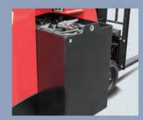
The battery side roll out is a part of the standard configuration. The truck can also be adapted to both BCI and BS standard batteries.
